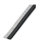
Taped ferrules, 1.5 mm<sup>2</sup>, sleeve length 8 mm, with plastic collar, according to DIN 46228-4, black, for processing with the CRIMPFOX 4 IN 1, 10 strips each with 50 sleeves per strip.
